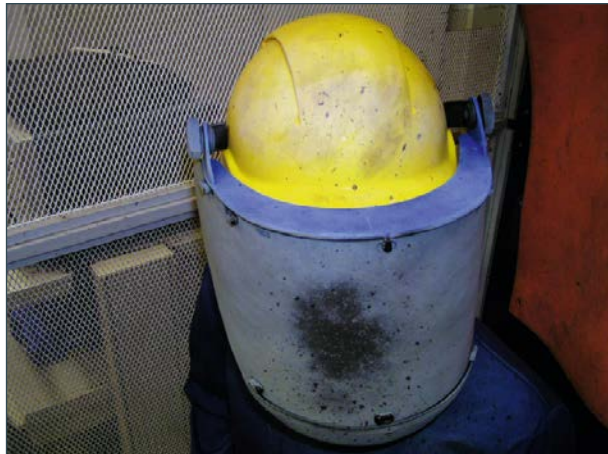
Our safety helmet for electricians with face shield protects the face and head region from injuries and burns.
